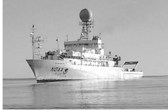
Figure 1. The C-band radar atop the central mast of the Ronald H. Brown research vessel.
