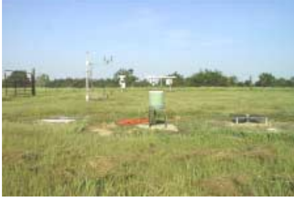
Figure 2. Station 50 in the center of the Goodwin Creek watershed hosting a variety of above-ground and buried rain gauges, raindrop disdrometers, wind profile measurements, and the SURFRAD station.
