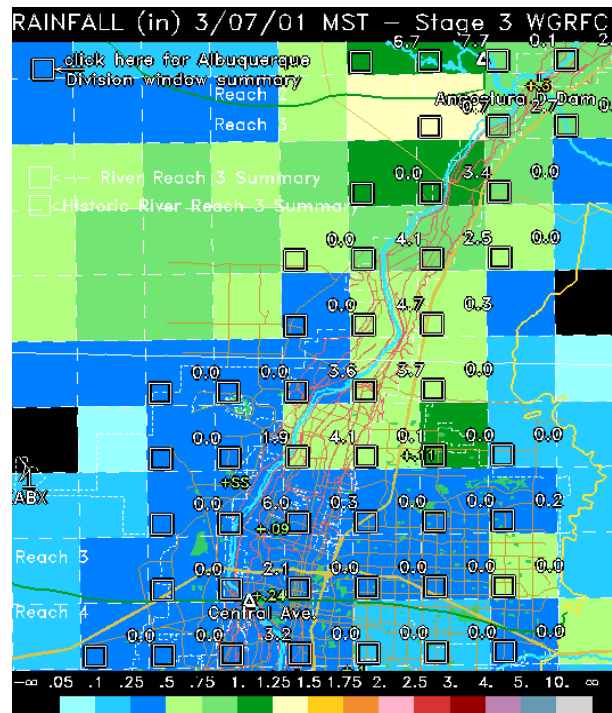
Figure 2. Example of an interactive image showing the grid cell 24-hr ET estimates and shaded 24-hr WSR-88D Stage III rainfall estimates.
