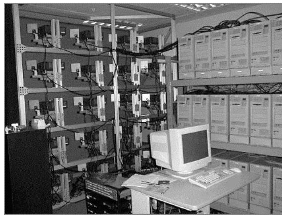
Fig. 3: The projectors behind the display wall mounted on a custom frame for adjusting the images so that they are continuous with minimum overlap.
