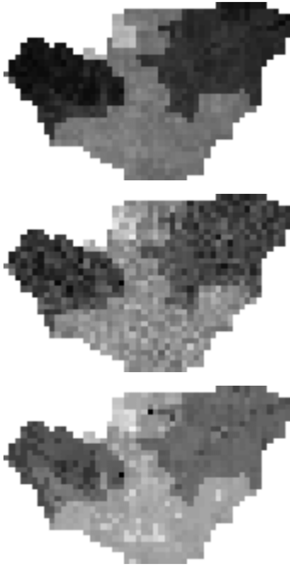
Fig. 4. DisaggNet soil moisture estimates for the dry soil case for 1.6 km (top) and 12.8 km (middle) aggregated emissivity input, compared to SHEELS 0-5 cm soil moisture (bottom). Light shading corresponds to low soil moisture, dark to high soil moisture.
