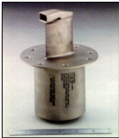
Figure 1. The WVSS sensor
