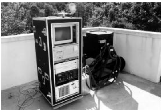
Figure 2 Photograph of the HARLIE transceiver assembly and electronics rack.
