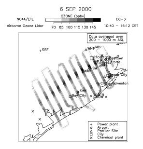
**Figure 3**: Horizontal distribution of vertically averaged ozone measured with the airborne lidar on September 6<sup>th</sup> between 10:40 and 16:12 CST. Note the different grey scale for ozone concentration as compared to Figs. 1 and 2.
