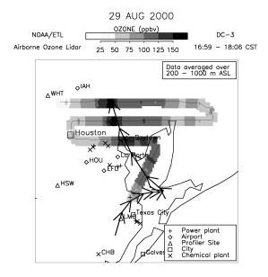
**Figure 1**: Horizontal distribution of ozone as measured with NOAA/ETL's airborne lidar along the DC-3 flight path on August 29<sup>th</sup> between 11:07 and 13:35 CST. Ozone concentrations are vertically averaged between 200 and 1000 m ASL. The sequence of arrows represents a back trajectory calculated from the wind profiler network data. Locations of the five wind profilers are indicated by triangles.
