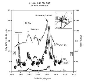
**Figure 4**: Traces of  $O_3$ ,  $NO_y$ ,  $SO_2$ , and formaldehyde measured with in situ sensors on board the Electra aircraft on the afternoon of September 6<sup>th</sup> during a flight transect downwind of the Houston urban area. Location of the flight leg is indicated in the inset figure. The flight altitude of the Electra was 650 m ASL.
