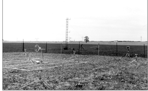
Figure 1: Gas source within windbreak, Elleslie, Alberta. Retro-reflector of methane laser is visible.
