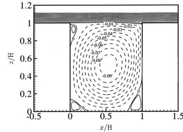
Figure 5: Spatial variation of the streamfunction. Positive (solid lines) and negative (dashed lines) streamfunction represent secondary (anticlockwise) and primary (clockwise) vortices, respectively. Streamfunction for the solid lines inside the three secondary vortices is equal to  $1.00 \times 10^3$ .
