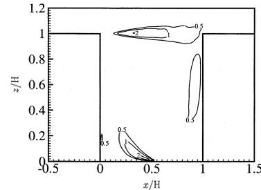
Figure 6: LES calculated spatial variation of the dimensionless vertical scalar fluxes  $\langle w''c'' \rangle (HL/Q)$
