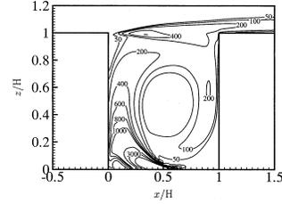
Figure 4: LES calculated spatial variation of the dimensionless mean scalar mixing ratio variance  $\langle c''c'' \rangle (UHL/Q)^2$  for  $x_s/H = 0.5$ .
