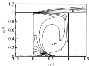
Figure 3: LES calculated spatial variation of the dimensionless mean scalar mixing ratio  $\langle \bar{c} \rangle UHL/Q$  for  $x_s/H = 0.5$ .
