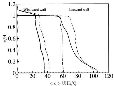
Figure 7: Dimensionless mean scalar mixing ratio on the windward and leeward walls for different source locations.  $x_s/H = 0.29$  (solid lines),  $0.5$  (dash-dotted lines), and  $0.71$  (dashed lines).
