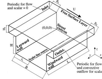
Figure 1: LES computational domain and boundary conditions for an idealized street canyon.
