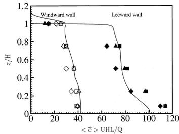
Figure 2: Dimensionless mean scalar mixing ratio on the windward and leeward walls. LES calculations: solid lines. Measurements: ■, □: Pavageau (1996), ▲, △: Meroney et al. (1996), and ◆, ◇: Pavageau and Schatzmann (1999).
