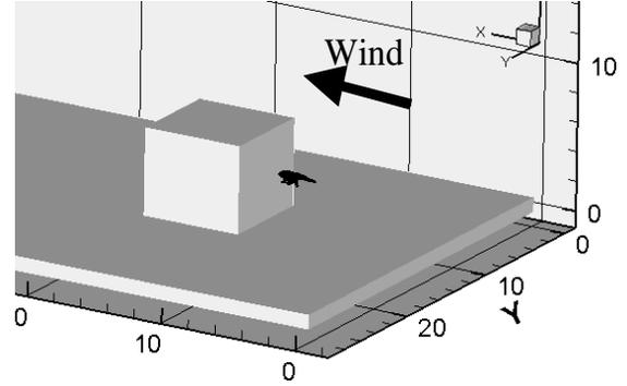
Figure 1. Particle trajectories for an upwind release 8 seconds after the release start time.
