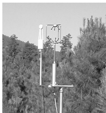
Fig. 2 Open-path eddy covarianc setup with a Gill Windmaster sonic anemometer and a Licor Li-7500 open-path IRGA.
