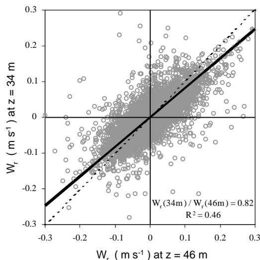
Figure 2: Comparison of the mean vertical velocity ( $W_r$ ) at 46 m and 34 m. The solid line indicates a principal axis linear regression (slope = 0.82). The dashed line indicates a slope of 1:1. (data from 1999)
