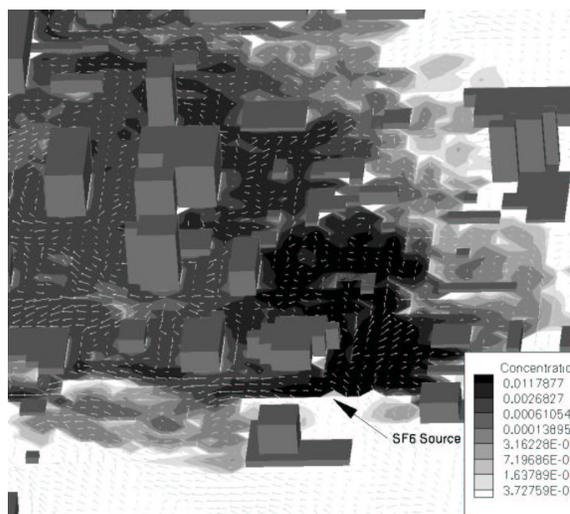
Figure 2: Wind and concentration fields at a height of 2.5m, near the source release point.
