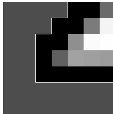
Figure 2: Kernel containing a plume-like shape for the wind direction shown in figure 1. Pixel values represent pixel coverage by the plume, except for the case of the black pixels. These have zero pixel coverage by the plume, but are set to negative values to offset the plume against its background and to give the kernel a mean of zero.
