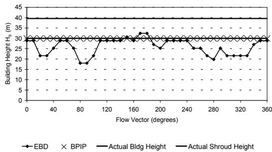
**Figure 2.** Building Height,  $H_b$ , predicted using the EBD technique, the BPIP program and the actual heights versus wind vector.
