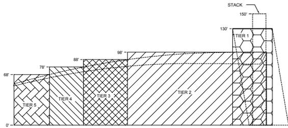
**Figure 1.** Simplification of the multi-tiered, porous, sloped structure for input into the BPIP program.
