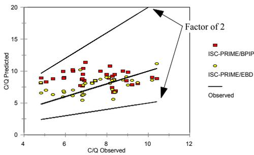
**Figure 3.** Maximum predicted concentrations versus those observed in the wind tunnel.
