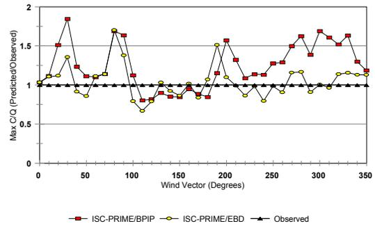
**Figure 4.** Maximum predicted and observed C/Q normalized by the C/Q observed in the wind tunnel versus wind vector.
