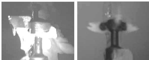
Fig. 5. Icing of IceFree II direction vane and speed rotor.
