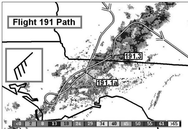
Figure 5. Path of Flight 191 and Tallahassee, FL Nexrad composite RRF (dBz) at 18:44:21 UTC. Flight level wind vector (knots) is in the inset. Bold black lines represent state borders of FL, GA, and AL. Severe turbulence encounters indicated on flight path.
