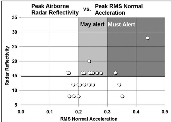
Figure 1. Comparison between  $\sigma_{\Delta n}$  and airborne RRF for 23 NASA turbulence events. RRF values greater than or equal to 15 dBz and  $\sigma_{\Delta n} > 0.20$  are alert threshold considerations for FAA radar certification.
