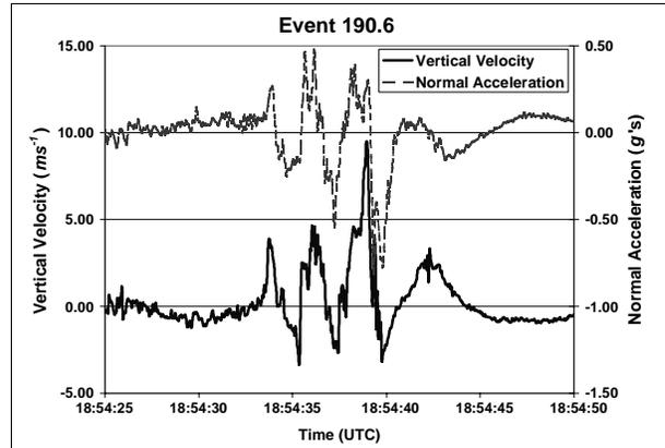
Figure 3. Plot of Vertical Velocity (solid line in  $\text{ms}^{-1}$ ) and  $\Delta n$  (dotted line in g's) for Event 190.6.
