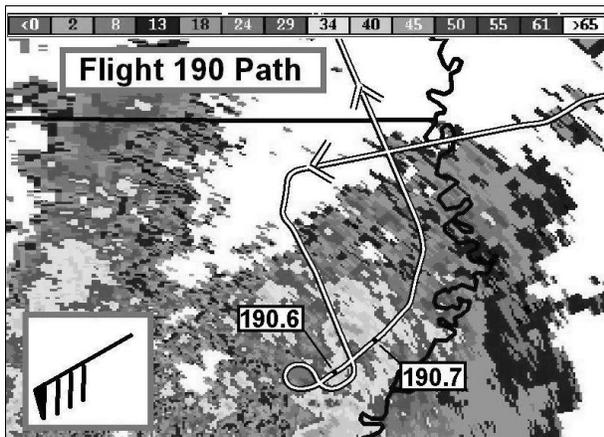
Figure 2. Path of Flight 190 and Fort Polk, LA Nexrad composite RRF (dBz) at 18:57:48 UTC. Flight level wind vector (knots) is in the inset. Bold black lines represent state borders of LA, MS, and AR. Severe turbulence encounters indicated on flight path.
