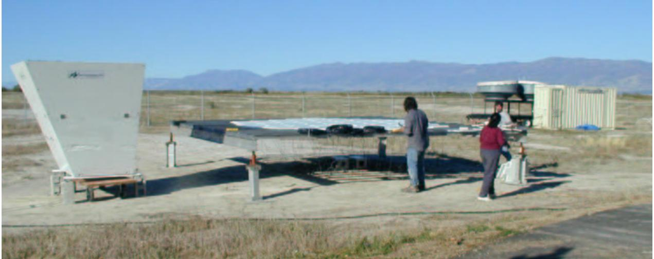
Fig. 1. University of Massachusetts students assembling the TEP receiving array, with the SODAR on the left, the FMCW-antennas on the right and the Wasatch Mountains in the background.
