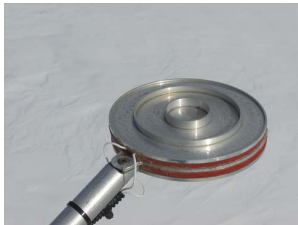
Figure 1 Top view of hotplate. Diameter of plate is 13.3 cm.
