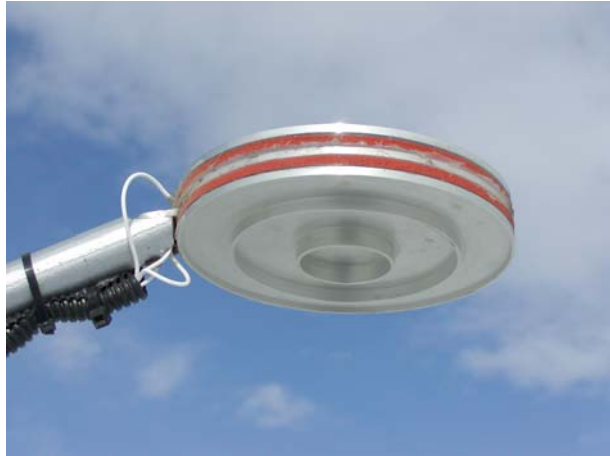
Figure 2 View of lower plate. Diameter of plate is 13.3 cm.
