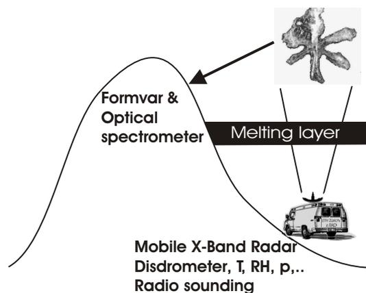
Fig. 1: Schematic drawing of the setup with two locations, one at the bottom and the second close to the top of the respective mountains.
