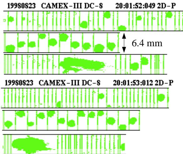
Figure 4: Large particle images observed with the NASA DC-8. The rejected images are in the third row following the strip label.
