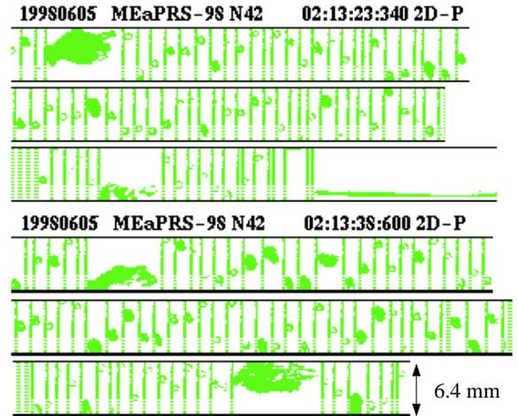
Figure 5: 2D-P images from a descent through a melting layer in a Midwestern MCS. Note the splash images in the first and sixth strips. These images were obtained at a temperature of  $+1^{\circ}\text{C}$ .
