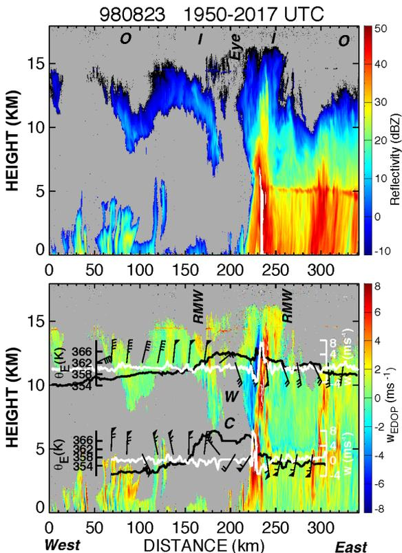
Figure 2. NASA ER-2 Doppler radar (EDOP) cross-section. The DC-8 and NOAA WP-3D vertical velocity and  $\theta_e$  are superimposed on the Doppler plot. Radar from Heymsfield et al, 2001.
