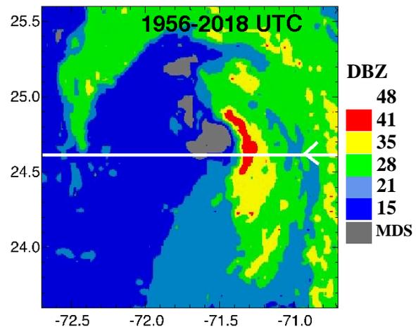
Figure 1: CAPPI at the 12 km altitude made from the NOAA WP-3D aircraft near the time of the ER-2 and DC-8 passes. The ER-2 flight track is shown. Adapted from Heymsfield et al, 2001.
