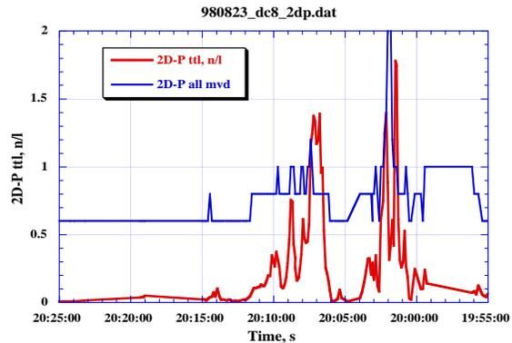
Figure 3. 2D-P Number concentration and Median Volume Diameter (MVD) from the NASA DC-8 2D-P. Data correspond to the radar data in Fig. 2
