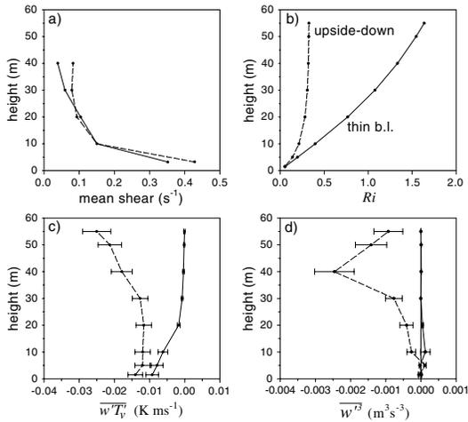
Figure 1: The composited vertical structure of the a) mean shear, b) local gradient Richardson number, c) virtual heat flux and d)  $\overline{w'^3}$ , for the class of thin traditional boundary layers (solid lines) and the upside-down class (broken lines)
