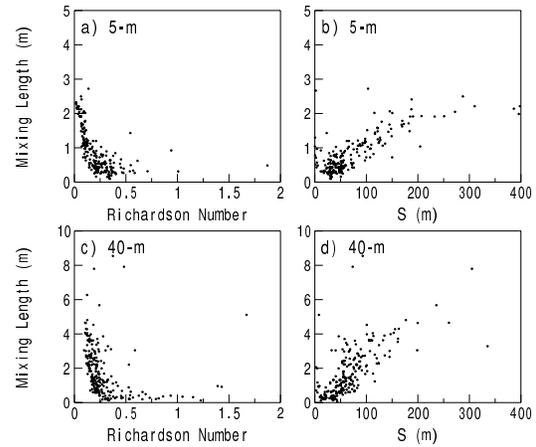
Figure 3: The dependence of the mixing length on the layer Richardson number centered about the eddy correlation level and the dependence of the mixing length on the bulk length scale (Eq. 2) for the 5- and 40-m levels.
