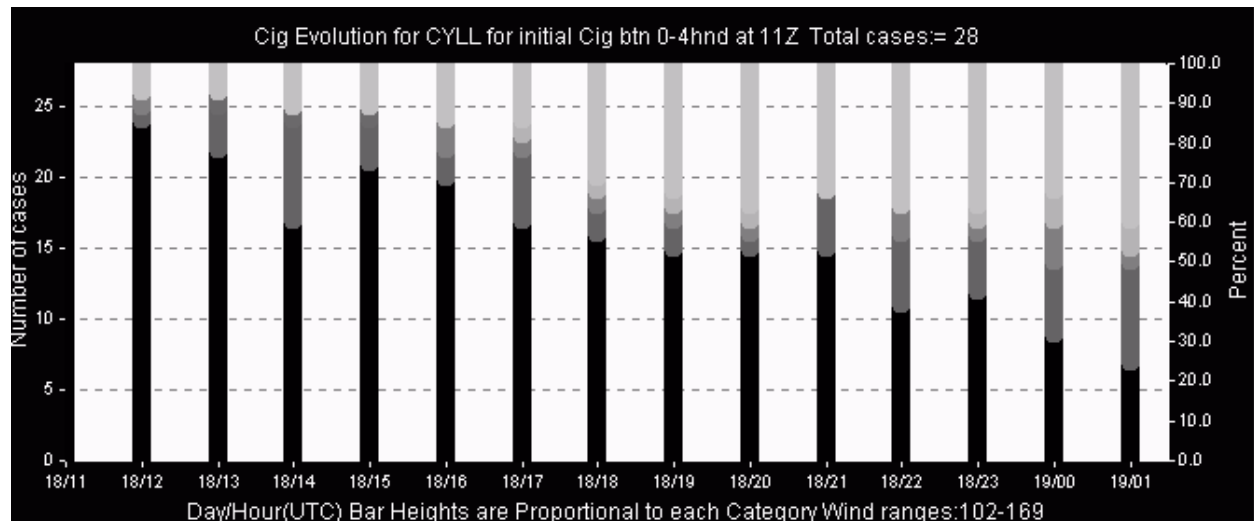
Figure 1. TAFaid conditional climatology output (the color version is easier to interpret). The forecast period extends from left to right, each bar representing one hour. The height of each segment within the bar indicates the probability of that particular ceiling category: IFR at the bottom of each bar, VFR at the top. In this particular case, for starting conditions between 0-4 hundred feet, with a southeast wind at 11Z, historically at least 50% of the cases remained between 0-4 hundred feet for 10 hours (until 21Z). As with most climatological tools, there is a tendency towards normal (VFR) conditions over time.
