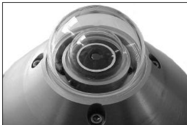
Figure 1. Close-up of the instrument without cover. The infrared detector is visible in the center of the receiver.
