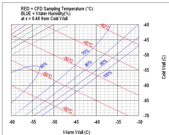
Figure 1. Continuous flow diffusion chamber aerosol processing conditions as a function of warm and cold cylinder temperatures in the processing regime used for most of this study. Figure courtesy of David Rogers (National Center for Atmospheric Research).
