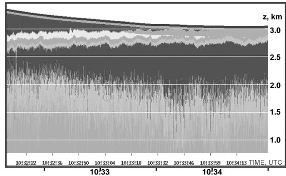
Fig. 1. Profile of altostratus layer over Lake Michigan on January 18, 1998 for 10:32 to 10:34 UTC obtained by SABL nadir lidar at IR wavelength onboard the NCAR Electra RF09 during Lake-ICE.
