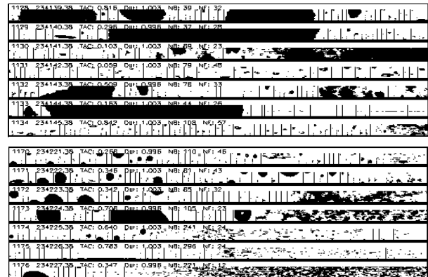
Figure 2: Images from the 2D-C probe in (top) the center of a radar-identified “hail” region more than 5 km across (visible dimension of largest particle about 1.2 cm), and (bottom) the adjacent updraft region with drops up to about 3 mm in size.
