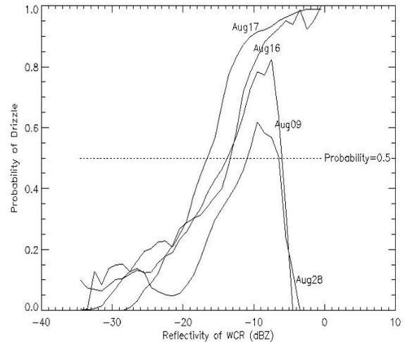
Fig 1. Drizzle's probability corresponding to different reflectivity values for 4 flight days.
