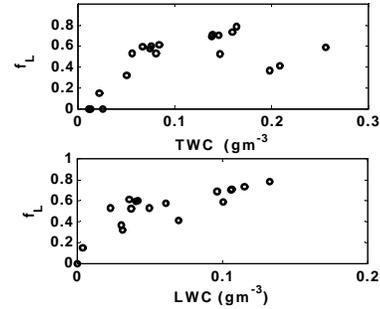
Fig. 3. The liquid fraction is plotted against the measured LWC and TWC with Nevzorov TWC/LWC probes. This data was corrected using Eq. 2.
