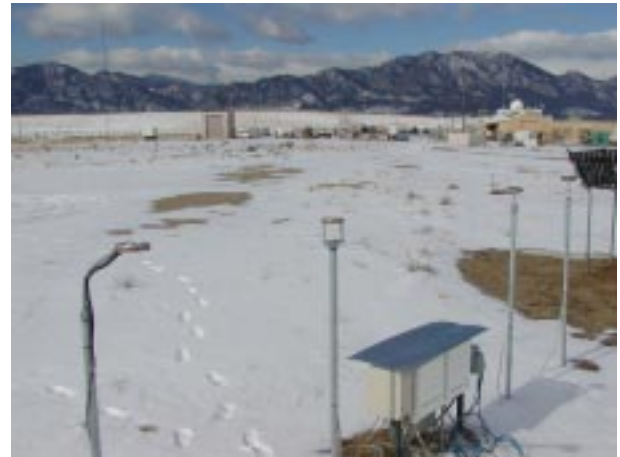
Figure 3 From left to right, “original” hotplate, Mt. Washington hotplate, coil hotplate, frisby hotplate. Left 1/3 of a half scale Wyoming shield is shown in the upper right of the photo.
