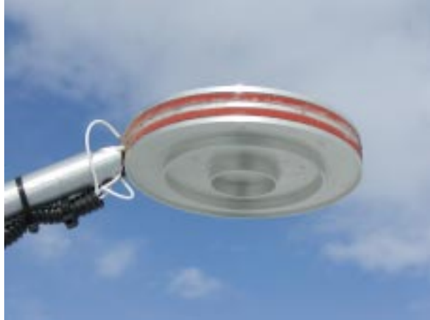
Figure 2 View of lower plate. Diameter of plate is 13.0 cm.
