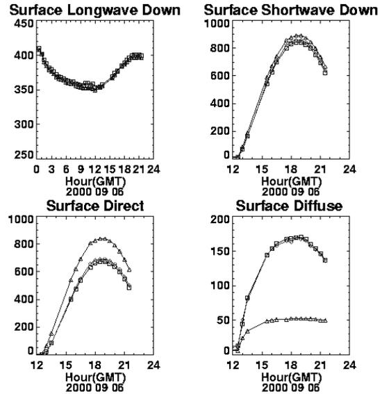
Figure 1. Comparison of observed (square) Fu-Liou model pristine (triangle) and model with observed aerosol (diamond) at ARM SGP for single day.
