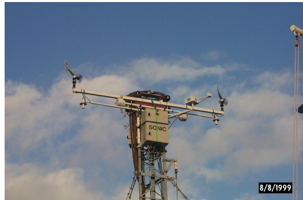
figure 1: Picture of the top of the instrumented mast. The meteorological sensors (anemometers, radiation sensors ...) and boxes create a lifting and a deceleration of the airflow.
