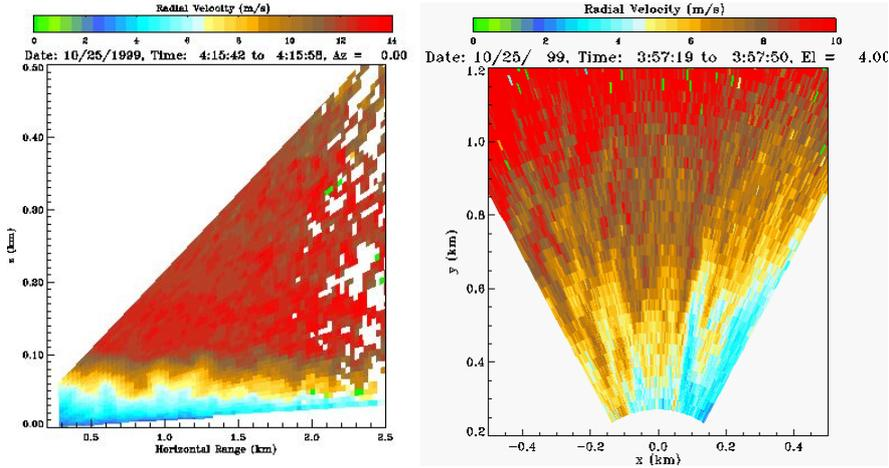
**Figure 3:** HRDL radial velocity field zoomed in the surface region (from earth's surface up to 500 m) retrieved from RHI scans (azimuth  $0^\circ$ ) at 0415 UTC (a) and from PPI scans (elevation  $4^\circ$ ) at 0357 UTC (b) on 25 October 1999. Positive (negative) radial velocities correspond to air blowing away from (towards) HRDL.
