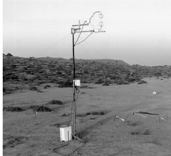
Figure 1. Eddy covariance flux station, at 3 m height
