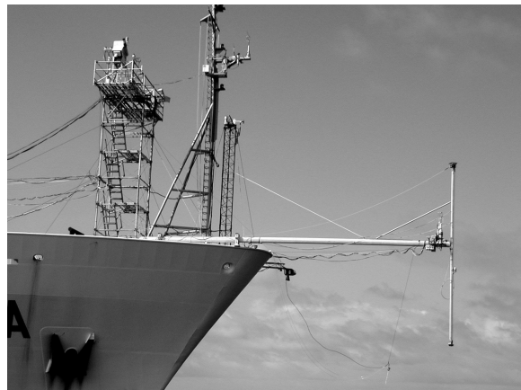
Figure 2. The boom extended 10 m from the bow. The 8-m mast extended from 4-12 m above the ocean surface.
