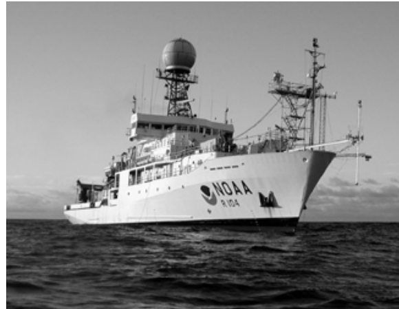
Figure 1. The NOAA R/V Ronald H. Brown outfitted with a bow boom and mast for the February 2001 GasEx experiment performed at 3S and 125W.
