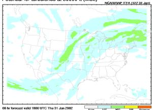
The ITFA output contains turbulence predictions ranging from none to extreme; higher values imply the likelihood of turbulence of a higher intensity. Table 3 provides an approximate correlation of the ITFA predictions to operational turbulence interpretations. A final determination of the relationship between ITFA predictions and operational interpretations will come after future intensive evaluations.
