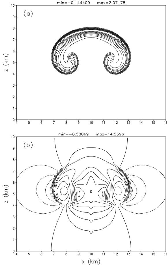
*Fig. 1 Results of the dry thermal simulation. (a) Perturbation potential temperature, contour interval 0.2 K, zero contour omitted. (b) Vertical velocity, contour interval  $2 \text{ m s}^{-1}$ , negative contours dashed.*
