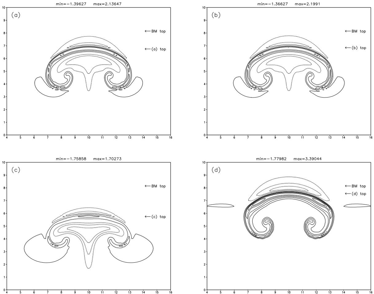
Fig. 3 Perturbation wet equivalent potential temperature from simulations using various model formulations: (a) equation set A, (b) equation set B, (c) equation set C, and (d) equation set D. Contour interval is 0.5 K. Negative contours are dashed. The zero contour is omitted. Near the right-hand side of each panel, the height of the top of the thermal is indicated, along with the height of the top of the thermal from the benchmark ("BM") simulation.
