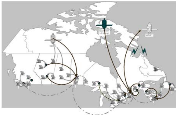
Figure 1: Data topology of the Canadian National Radar Network. The radar icons indicate the location of the radars. Solid lines indicate existing pathways for the volume scans and the dashed lines indicate future radar installations. Dash-dot lines indicate inter-Regional data flow paths. Note the ingest of NEXRAD data at the Canadian Meteorological Centre and the subsequent re-transmission to the Regions via SATNET.
