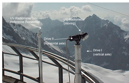
Fig.1: Measuring system ASCARATIS at mountain Zugspitze
