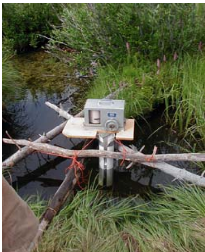
Figure 2: Recording flow meter.
