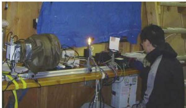
Fig. 2. Atmospheric Sciences graduate student Dong-Chul Kim calibrating a UV actinic flux sensor prior to field deployment.
