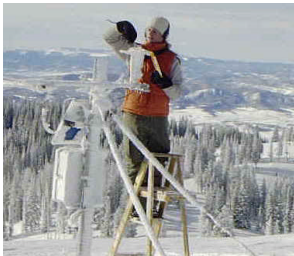
Fig. 3. Hydrologic Sciences graduate student Katrina Smolen working with tower instrumentation system for characterizing the radiative energy budget of an open snowfield.
