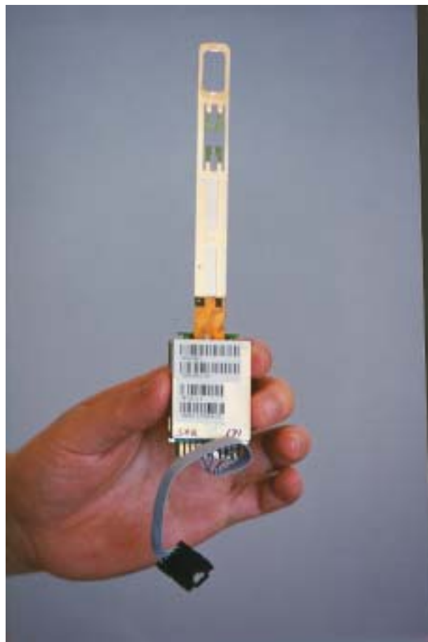
Figure 2: Vaisala RSS901 PTU sensor mounting on Aerosonde
