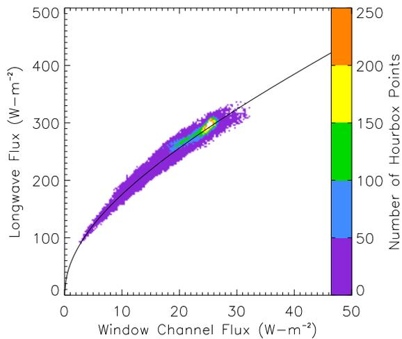
Figure 6. Histogram of OLR versus window channel flux and curve fit for India region, January 1998.
