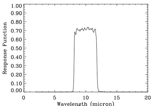
Figure 1. Spectral response of CERES 8-12  $\mu\text{m}$  window channel.
