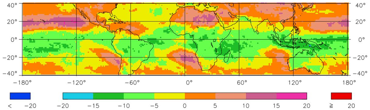
Figure 5. Map of difference between OLR as measured by broadband channels and as inferred from window channel for January 1998,  $W\cdot m^{-2}$ .
