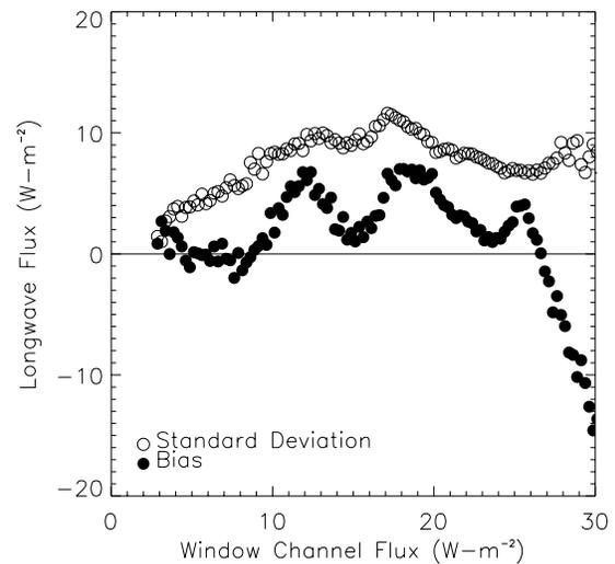
Figure 7. Bias and standard deviation of OLR derived from window channel measurements using curve fit for India region, January 1998.
