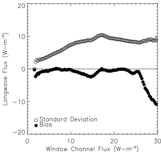
Figure 3. Bias and standard deviation of OLR derived from window channel measurements using curve fit for all TRMM coverage area, January 1998.
