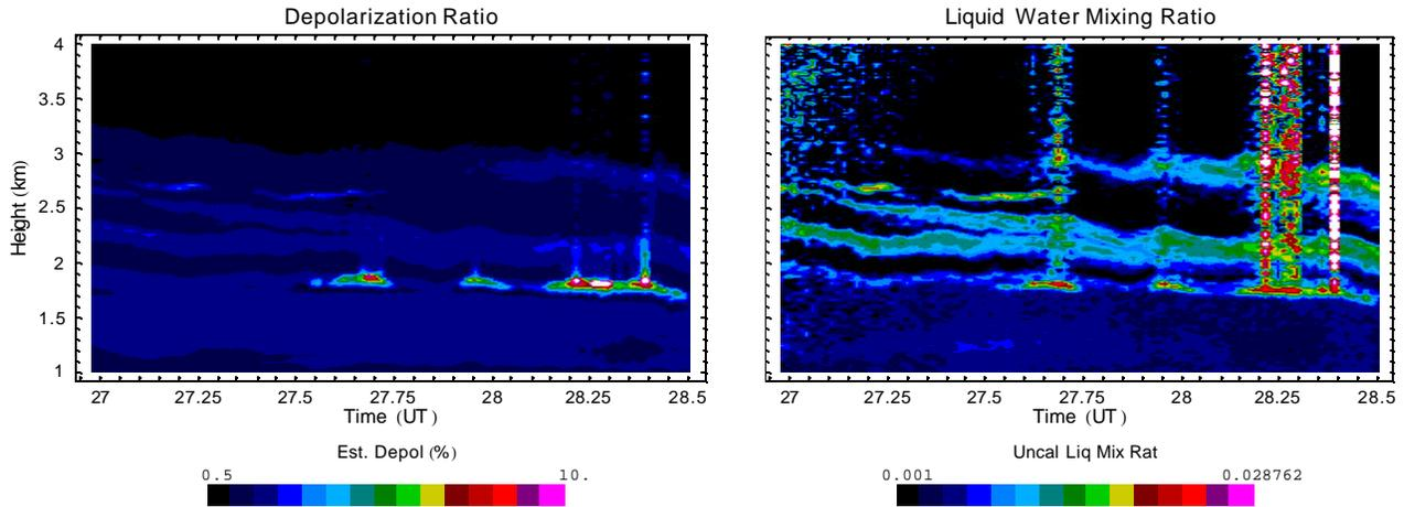
**Figure 2** Aerosol depolarization and liquid water mixing ratio (uncalibrated) measurements from the night of May 25, 2002 during the IHOP field campaign. The high correlation between the aerosol layers and the liquid water signal is evident. The strong scattering from aerosols (in addition to the previously measured liquid water in clouds) points toward a new technique for measuring the liquid water content of aerosols in the atmosphere.
