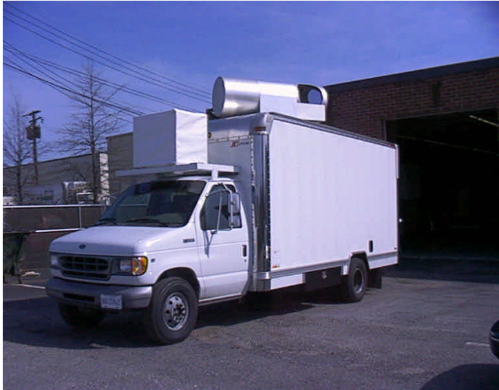
Figure 1 The mobile Doppler lidar system is mounted in a modified delivery van. The 45 cm clear aperture azimuth-over-elevation scanner is mounted on the roof to allow full sky access.
