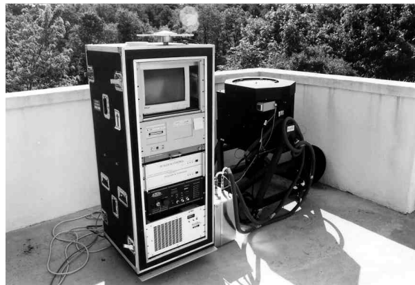
Figure 2 Photograph of the HARLIE transceiver assembly and electronics rack.
