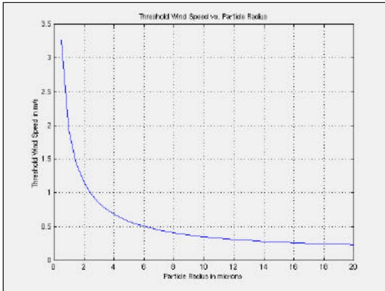
**Figure 3** Dust threshold surface wind velocity calculated in CARMA using the method described by Iverson and White [1982]. Notice that smaller size dust grains require higher surface wind speeds to mobilize since they are embedded in the soil matrix until liberated by larger particles.
