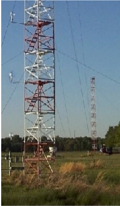
Figure 1. Photograph of the ARL 30meter met tower at Blossom Point, MD. 3D sonic anemometers are mounted on the tower
