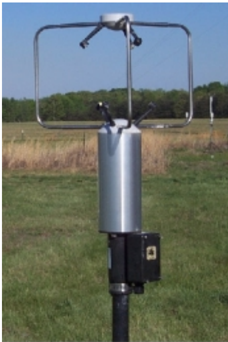
Figure 2. RM Young 3D ultrasonic anemometer (no moving parts)
