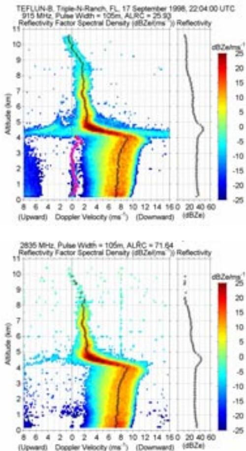
**Figure 3.** Spectral density plots for 915 MHz profiler (top) and S-band profiler (bottom) for observations taken simultaneously during stratiform rain on 17 September 1998 during TEFLUN B. Note the Bragg returns at the lowest heights in the top panel that are largely missing in the bottom panel.
