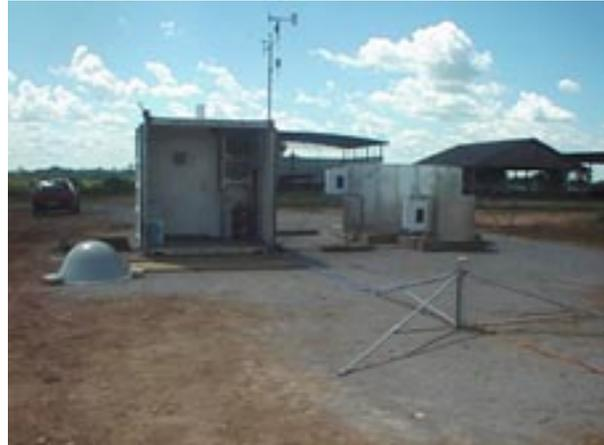
**Figure 1.** Low-powered S-band profiler antenna in front of the larger 915 MHz profiler antenna located at Ji-Parana airport during TRMM LBA.
