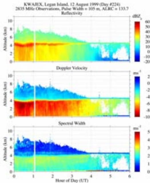
**Figure 7.** A 6-hour cross section of equivalent reflectivity, Doppler velocity and spectral width recorded at Legan during KWAJEX.
