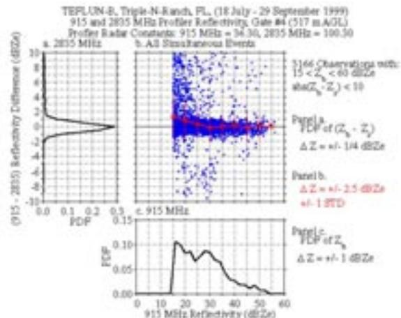
**Figure 4.** Scatter plot showing reflectivity differences (915 MHz – 2835 MHz) between the two collocated profilers located in central Florida during TEFLUN B as a function of 915 MHz profiler reflectivity.
