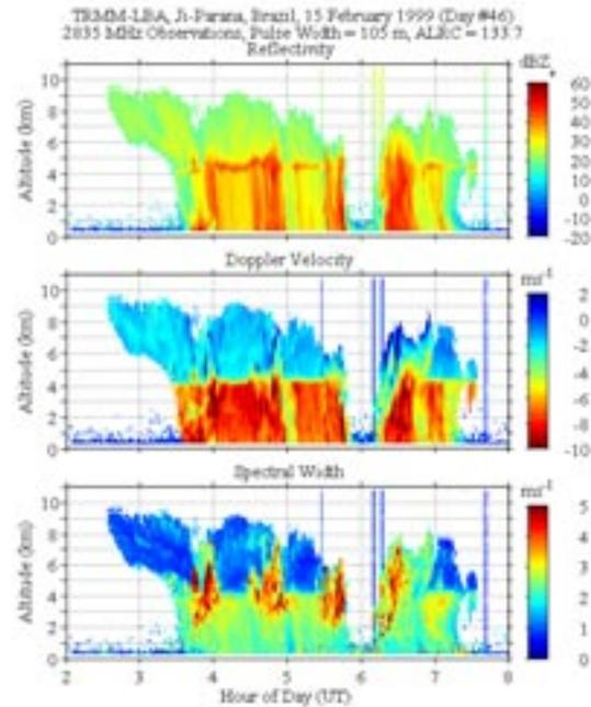
**Figure 6.** Equivalent reflectivity, Doppler velocity and spectral width associated with a nocturnal mesoscale convective system passing over the profiler at Ji-Parana, Brazil during TRMM LBA.
