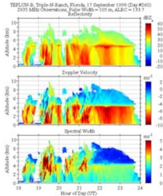
**Figure 5.** Equivalent reflectivity, Doppler velocity and spectral width associated with a mesoscale convective system passing over the profiler at the Triple N Ranch during TEFLUN B.
