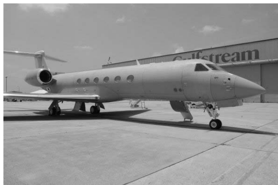
Figure 1. The "green" (basic) HIAPER airframe, a Gulfstream V (G-V) business jet.
